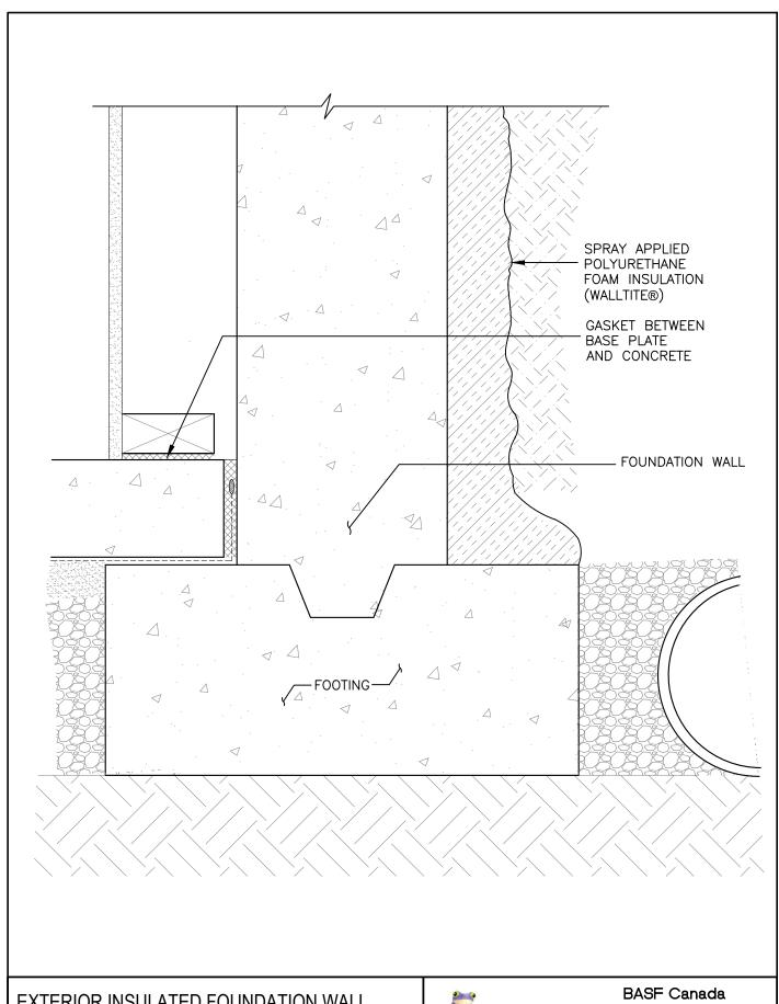
EXTERIOR INSULATED FOUNDATION WALL - BASEMENT
